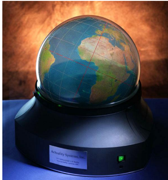
Figure 10: Perspecta - First commercial volumetric display; photomontage ( www.actuality-systems.com )
