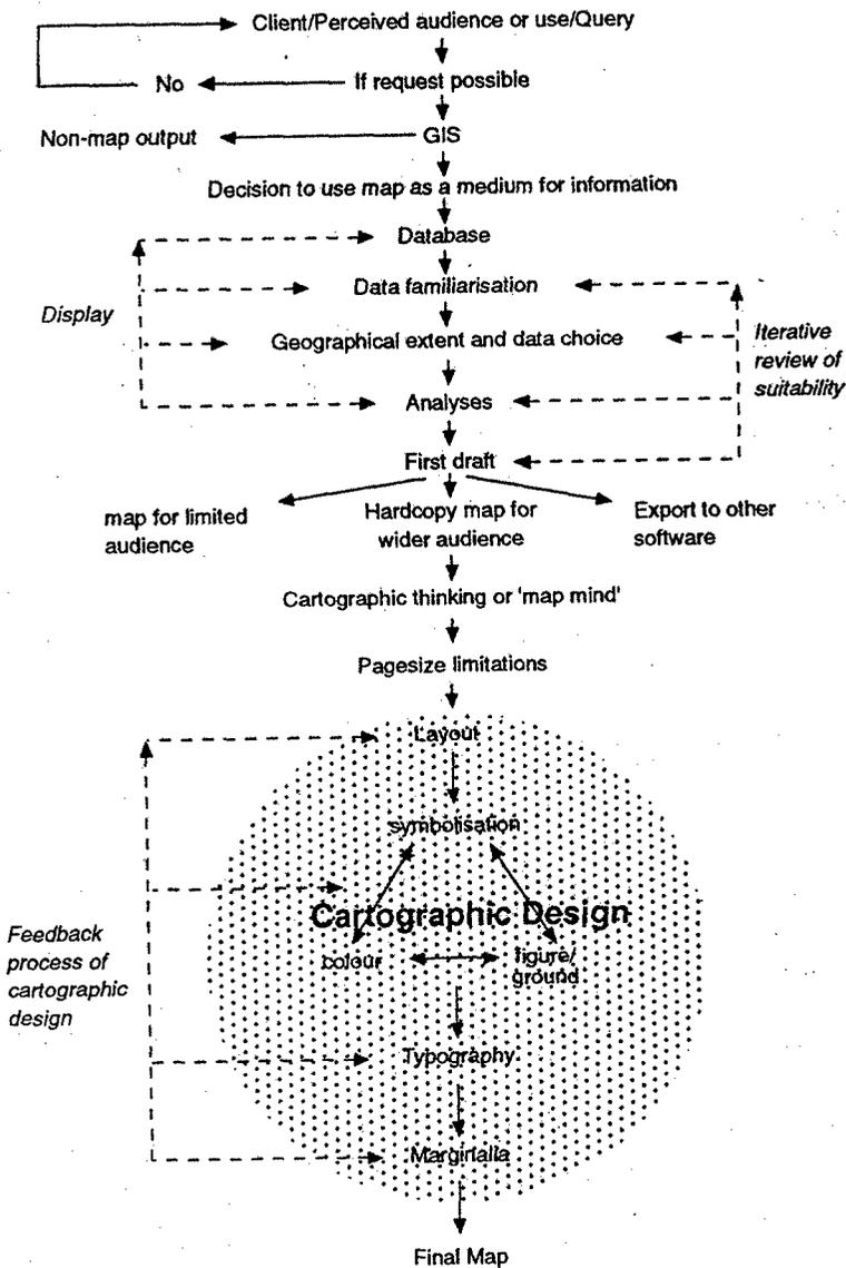
Figure 1. Idealised model of hardcopy map output for multiple users from a GIS.
