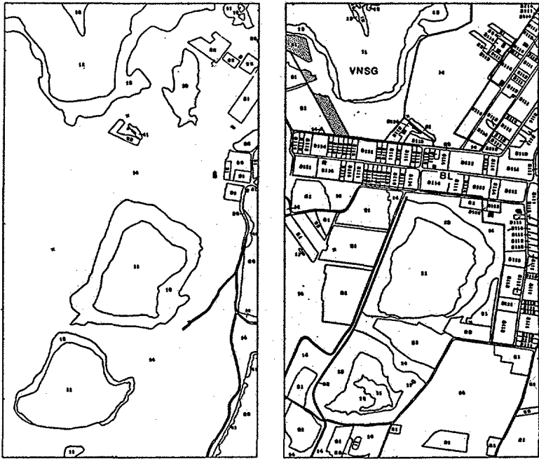
Figure 3: Test site Illmitz/Kirchsee, digital maps of landcover 1957 (left) and 1985 (right), aerial photo-interpretation with analytical plotter, map scale 1:10000 reduced to M \approx 12500 [7]. Classification key: 11 - water, 12 - littoral, 13 - reed, 14 - grazing lands, 21 - vineyards, 22 - fields, 31.. - housing (VNSG - primary zone of national park, BL - residential)
