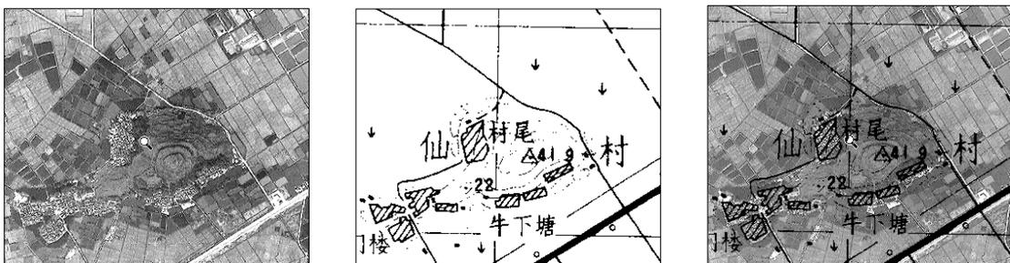
Figure 1a Overlaying DRG with rectified image (no partial distortion)
