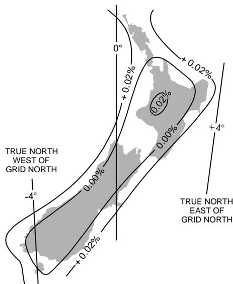
**Figure 6.** Scale error and convergence for the New Zealand Grid Projection.
