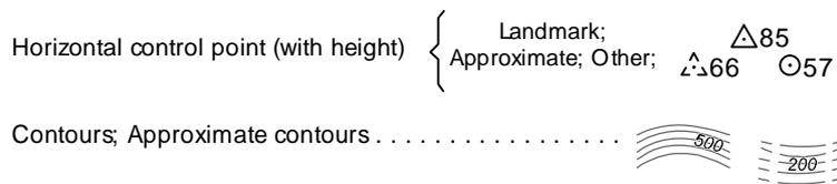
**Figure 3.** Symbolisation of reliability on a topographical map. Source: Central Mapping Authority of NSW, 1982.
