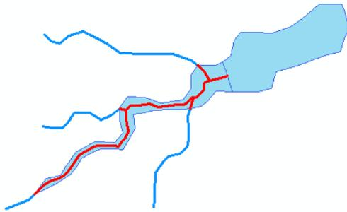
Figure 4c. Centerline and connecting lines created automatically.
