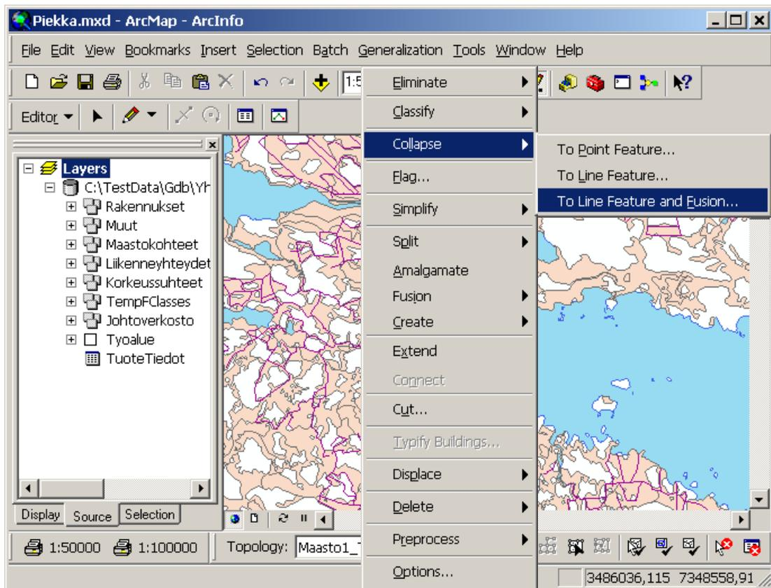
Figure 2. The Generalization menu provides the core edit commands for database and cartographic generalization.
