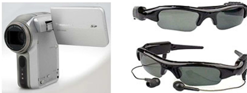
Fig. 2: Camcorder Panasonic SDR-S100 (left) and Mobile Eyewear Recorder (right) for video and audio recording.
