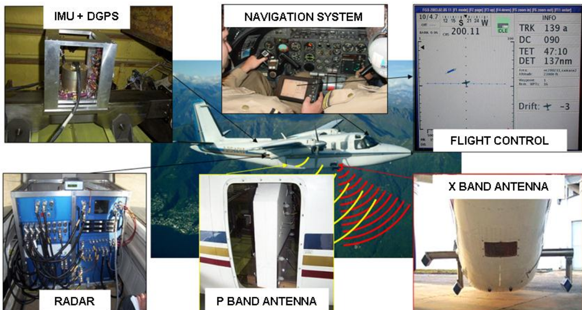
Figure 2 - Equipment used in the imaging system OrbiSAR RFP-airborne (flight segment).
