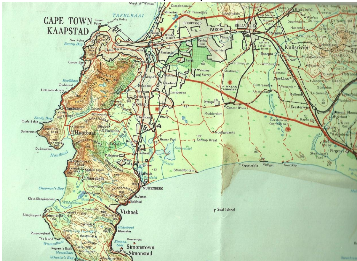
(Figure 6) Part of 3318 Cape Town, 3rd edition. Surveyed and drawn 1954, printed 1965. Uses the lilac grey fill for built-up areas. In the style laid down in the 1963 specification. Original scale 1:250,000
