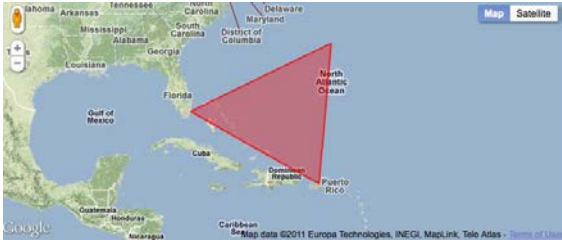
Figure 14.14 The Google Polygon function draws a closed shape. Options include strokeColor, strokeOpacity, strokeWeight, fillColor and fillOpacity. (© 2014 Google)
