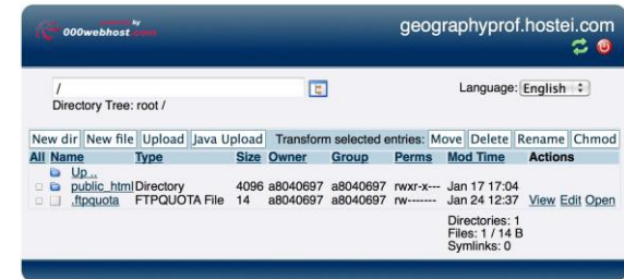
Figure 14.3 shows the File Manager Window from an online hosting service. This service allows files to be created and edited. All files to be served through the web must be in the public_html directory/folder. (© 2014 First Class Web Hosting)
