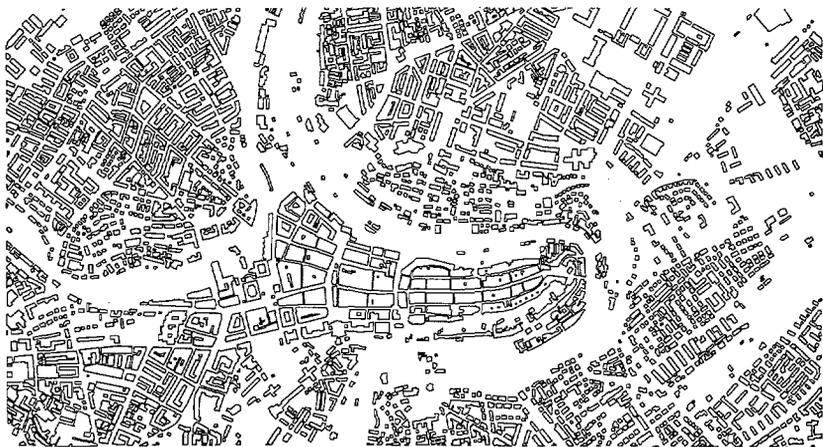
Fig. 6: Automatically extracted buildings, city centre of Bern (Switzerland), vector data (DXF).
