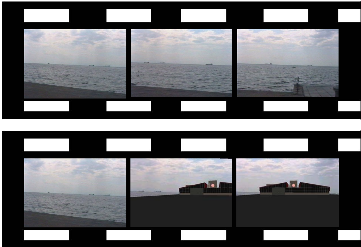
Figure 2. Mixed Reality for viewing a projected development: the 3D file of a new building is inserted in the video sequence displaying the existing situation. Above: frames from a video showing the current status. Below: video fused with the 3D display.
