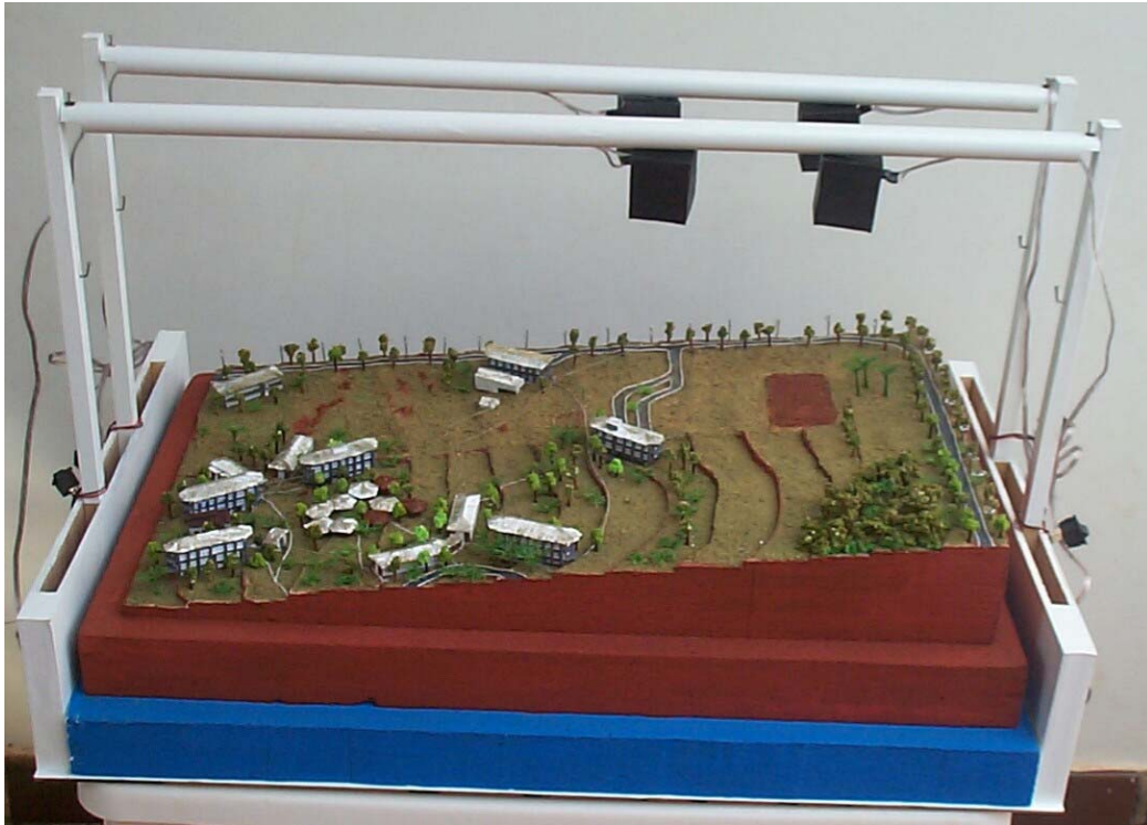
Photo 3: Model of simulation of an aerophotogrammetric survey.
