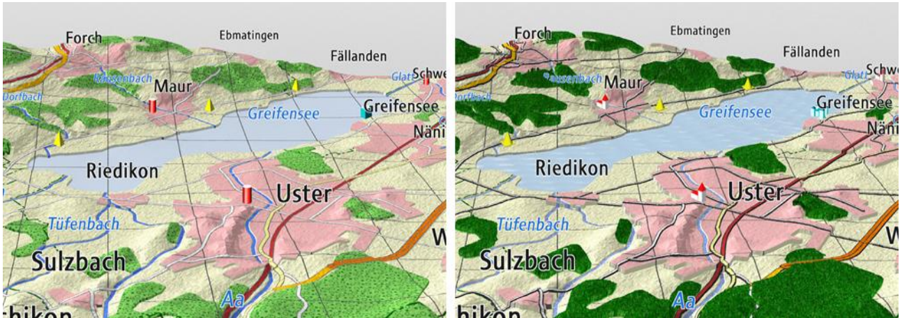
Figure 3: Examples of a topographic 3D maps, computed with symbolized vector data. Left: cartographic symbolization with a high abstraction degree; right: cartographic symbolization with a moderate abstraction degree (Haeberling 2004).
