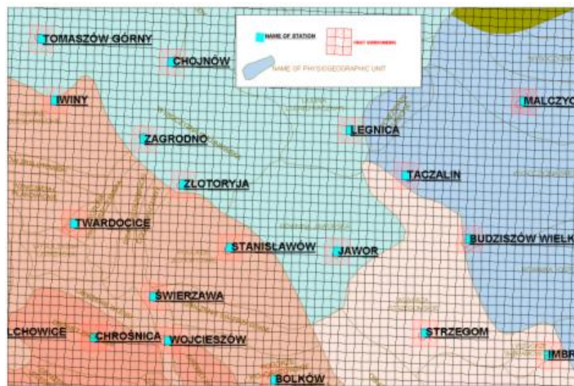
Figure 3. Grid of about 1 km sq.; measured points and physiogeographic units by Kondracki
