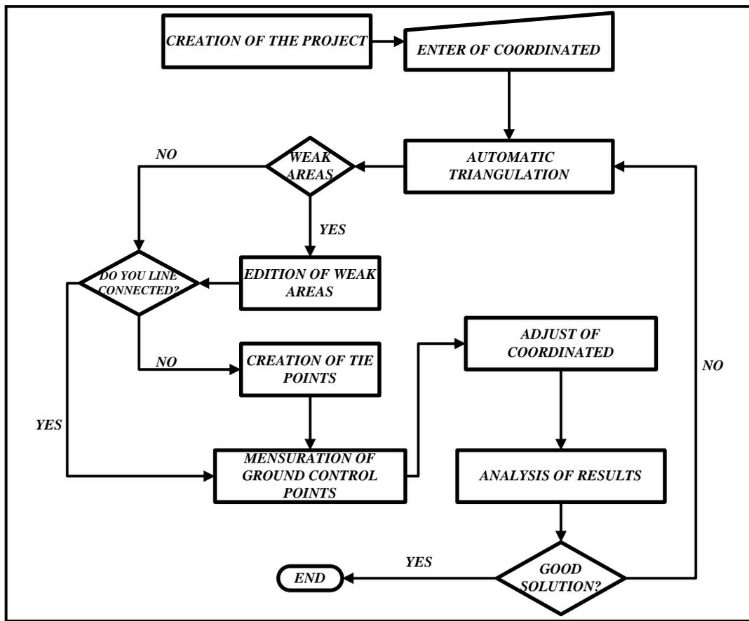
Figure n°1 'Digital spatial triangulation workflow'
