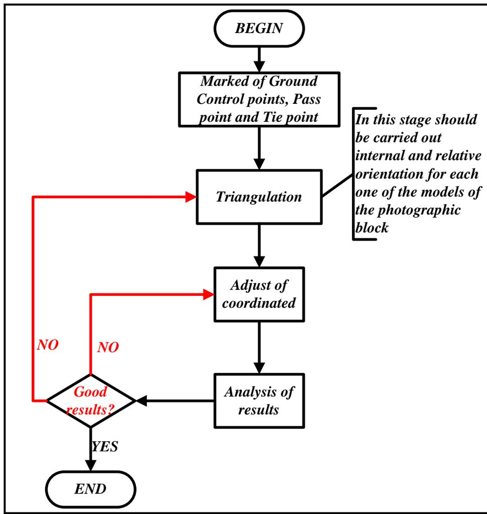
Figure n°1 'Analytic spatial triangulation workflow'
