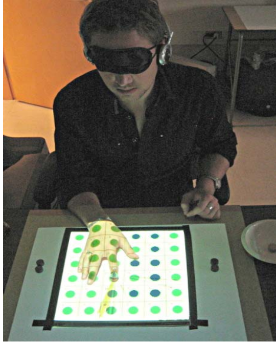
Figure 1: A participant with simulated vision impairment explores a test scene using the Fuse-Map Prototype. Target points are shown in blue.
