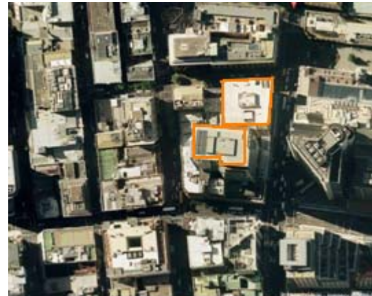
Figure 3. The highlighted areas show two multi stories building on an ortho-aerila image. As it can be seen, the taller building covers the neighbourhood areas. This issue is originated from degraded object regarding to the high and depth of view.
