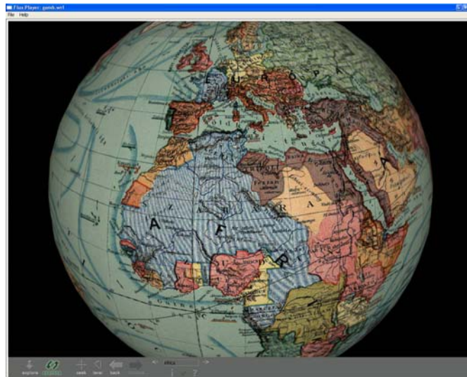
Figure 6: Moiré effect appearing due to and interference of the sampling grid and the printing raster
