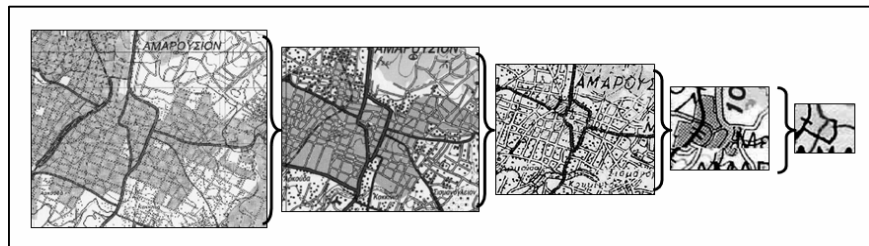
Figure 2. Examples of generalization techniques in polygons cartographic objects (Greek topographic maps from 1:25.000, 1: 50.000, 1:100.000, 1:250.000 1:500.000, Pantazis et al., 2008)
