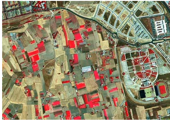
Figure 3: SPOT5 image from the PNT 2005 coverage. Infrared false colour. Pixel size 2,5 m (“Pansharpened”).
