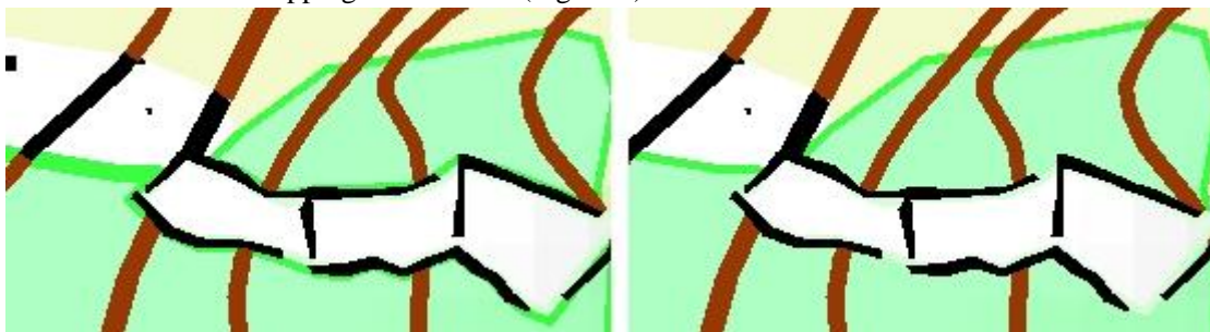
Figure 7: Application of symbol levels (left: without, right: with levels) in order to suppress forest contours in rock areas
