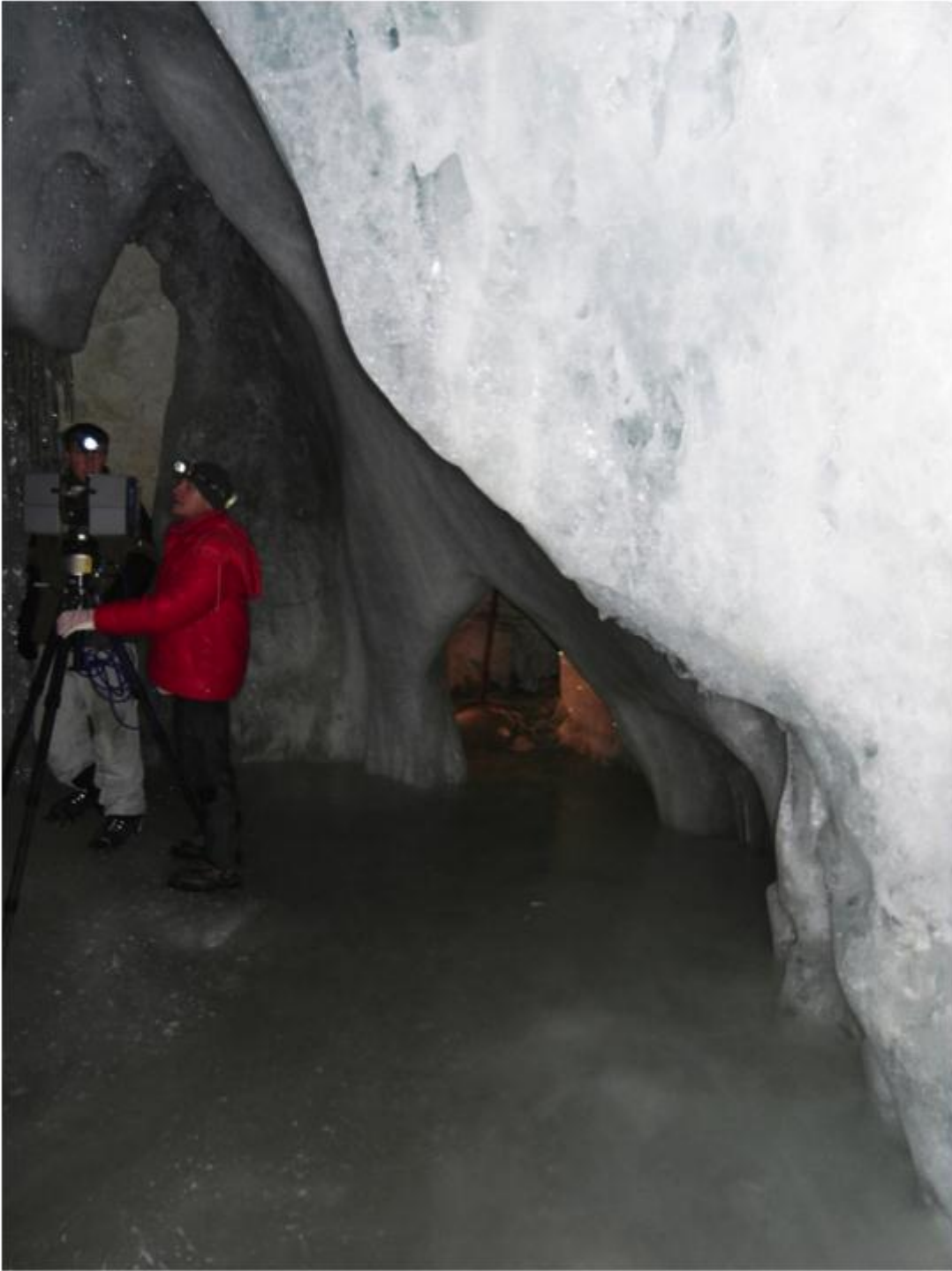
Figure 4: Some portions of the Eisriesenwelt represent real labyrinths of ice. A multitude of TLS scans are required to reflect the real-world conditions.
