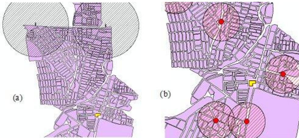
Fig 3.8. Buffers at a 500m distance from high voltage pillars (a) and 200m distance (b) from the location of gas stations. The user can see that the facility is located safely outside the restricted buffers.
