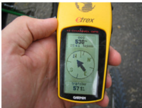
Figure 2. Typical eTrex operation showing direction of waypoint from current position
