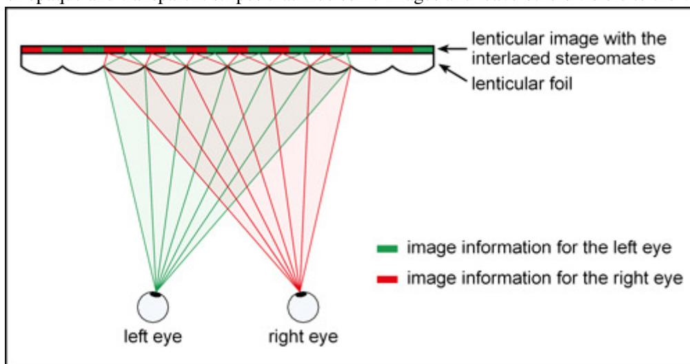
*Fig. 1: Principle of the lenticular foil technique*
