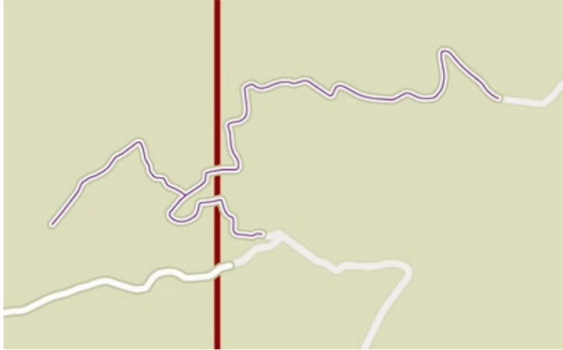
Figure 5: The Check Isolated Groups tool produces output features that identify isolated collections of roads after processing with the Thin Road Network tool. The vertical red line is a partition boundary.
