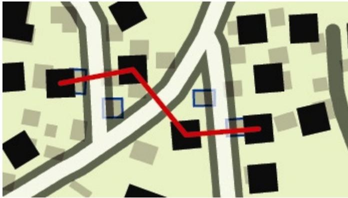
Figure 3: The original size, shape, and location of the four identified buildings before processing with the Resolve Building Conflicts tool are shown with a blue outline. The arrangement of these four buildings after processing has been identified with a red line by the Check Spatial Relationships tool. In this case, the results could be valid as the two acute angles of the roads force the buildings near the apexes to be moved significantly away from their original locations in order to meet the minimum size and minimum spacing requirements.
