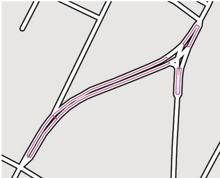
Figure 9: The pink polygons created by the Detect Line Overlap tool indicate areas in the output of the Merge Divided Roads tool where parallel, equal classification roads remain unmerged.
