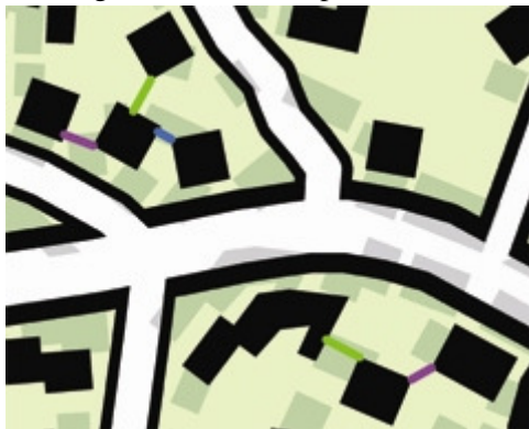
Figure 7: The Check Minimum Gap tool identifies features that are too close together, based on a distance parameter. In this example, only building-to-building distances were assessed, using a minimum distance of 15m apart. Green lines indicate very minor infractions, where two buildings are within 95% of the allowable distance, between 14.25m and 15m. Purple lines indicate infractions of the minimum distance that are between 50% and 95%, where buildings are between 7.5m and 14.25m apart. Blue lines show the most severe infractions, where the distance between buildings is less than 50% of the minimum allowable distance, or less than 7.5m apart.
