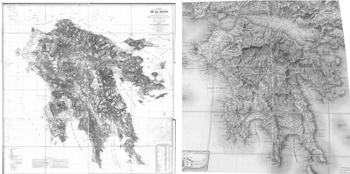
Figure 2. Left: The Expédition map (1828-1832) in the equivalent Flamsteed map projection. Right: The projection alteration of the Lapie 1826 map when best fitted in the Expédition map according to a second order polynomial transformation.
