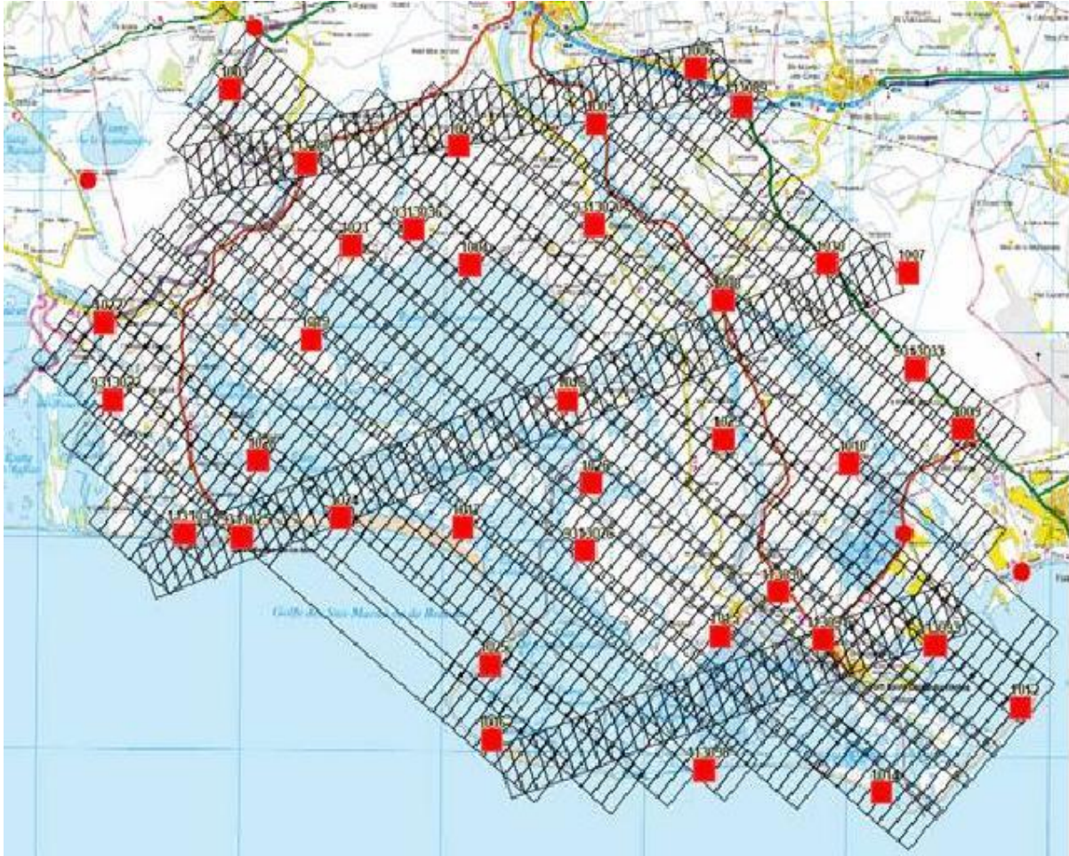
Figure 4: flight plan on the Rhône outlet including cross strips (the square dots represent the control points)
