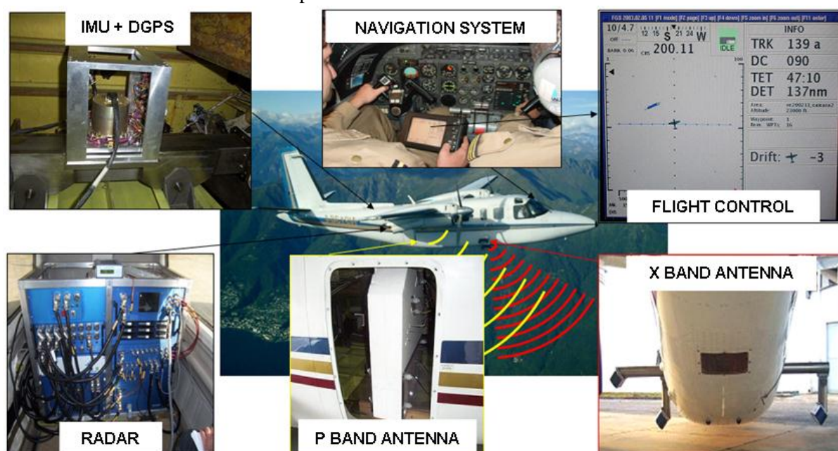
Figure 2 - Equipment used in the imaging system OrbiSAR RFP-airborne (flight segment).
