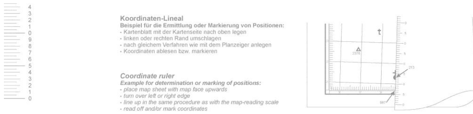
Figure 4: Coordinate ruler description with 2 millimetre lines at the rear side of the map
