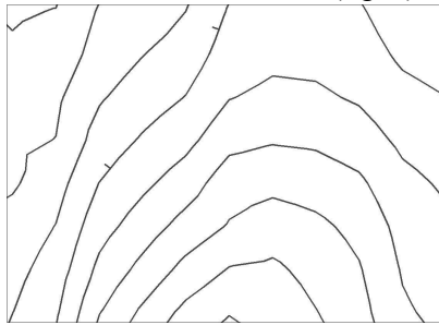
Figure 2. Set of contours with down-slope indicators
