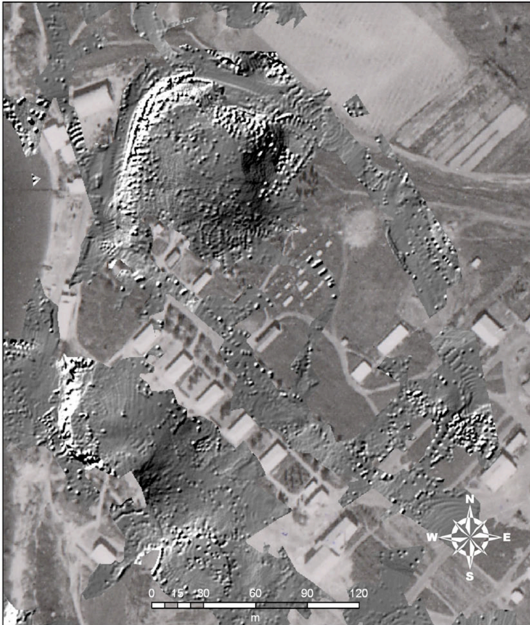
fig.2 Relief map generated from DSM overlaid on aerial photo
