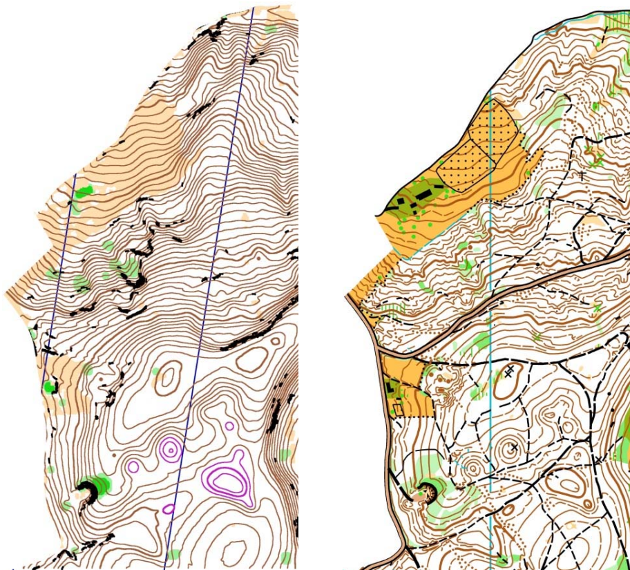
Figure 6. Automated created O-map and corresponding O-map, made for lidar data, too, from hilly, partly karstic area near Maribor
