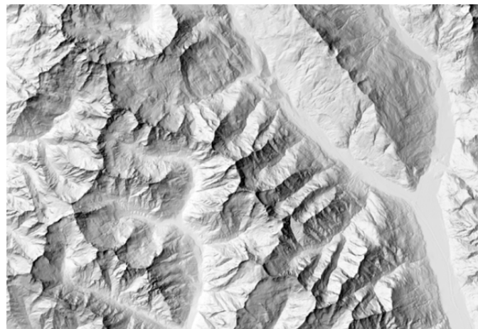
Figure 9. Shaded relief generated using the ArcGIS Hillshade function combined with the aerial perspective effect calculated within watersheds, complemented with light changes within watersheds and the two light sources originating from the Northwest ( 315^\circ ) and West ( 280^\circ ).
