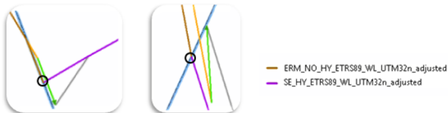
Figure 16. Adjusted features are connected on the border.
