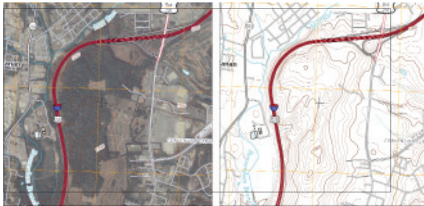
Figure 2. Portion of the Hollidaysburg, PA US Topo product with the image layer on (left) and off (right).
