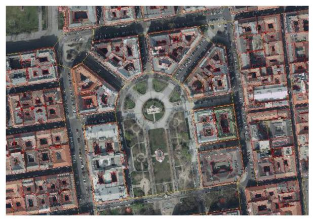
Aerial and space-born remote sensing data, point-clouds and special orthoimagery derived from point clouds, automatically generated LOD2 building models for cadastral data monitoring and update
