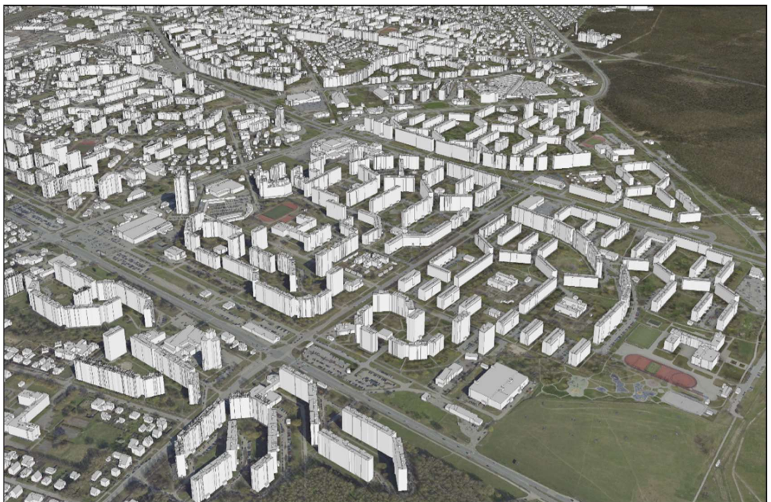
The vectorized LOD 2 model for the territory of Riga, prepared from airborne laser scanning data obtained in 2021
