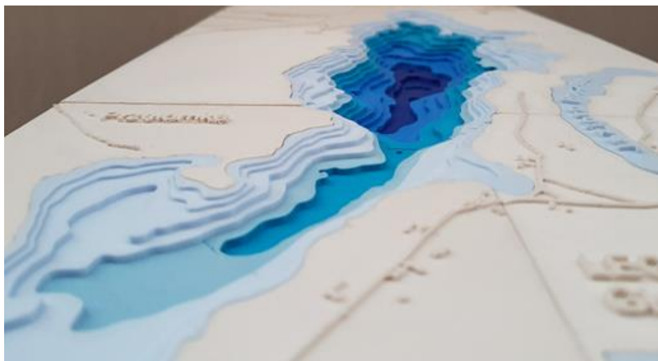
Fig. 61. 3D printed Bathymetric Map of Hańcza Lake done as part of engineering thesis (Source: Milewska A., Development of a bathymetric map using 3D printing . Engineering thesis, WAT 2019, Warsaw)
