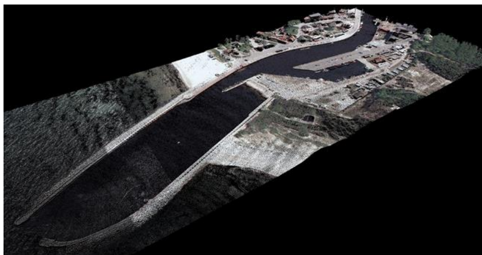
Fig. 5. Example of point cloud visualized by RGB values
