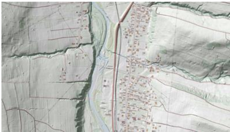
Fig. 6. Example of DEM data with superimposed topographic objects
