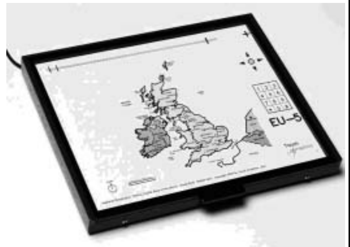
The Talking Tactile Tablet (TTT or T3), with a sheet from the National Geographic Talking Tactile Atlas of the World mounted.
