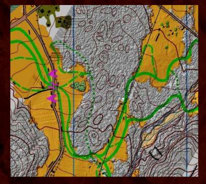
SKI-O map 8 sq.km DTK5 DEM 0.5 m DSM 5 pt/m2 orthophoto 0.5 m GPS (ratrac, scuter) 2 hours field check
